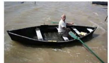
Trow rowed with copsed oars & thole pins
